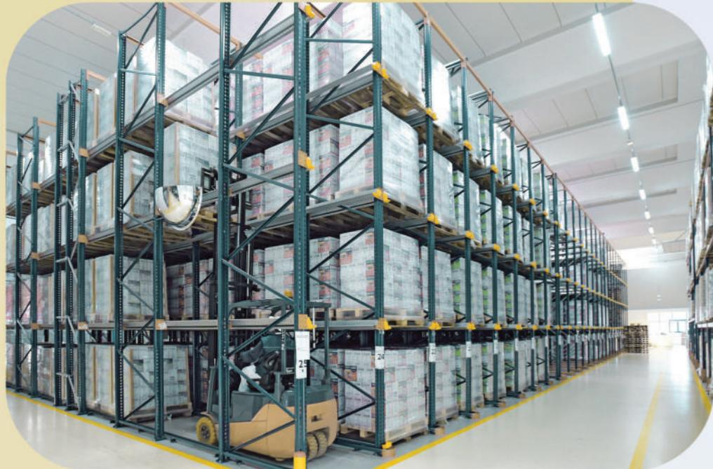
This system is totally similar to Selective Pallet Racking with deeper & double spaces then the fork lift can drive in through the system to organize the goods.
